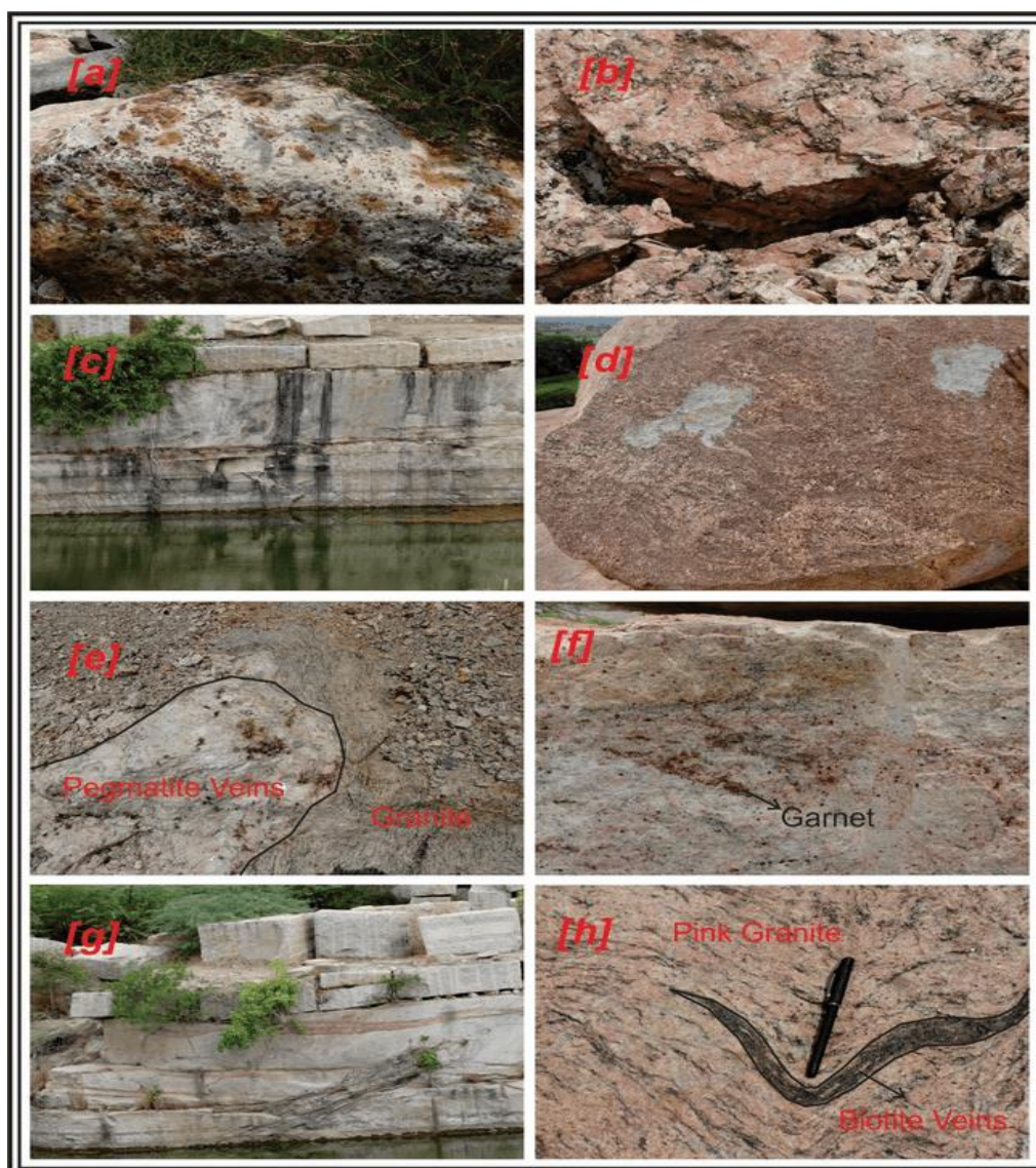
Figure 3: Field photographs showing in (a) Leptynite (Kashmir White) is a product of remelting of the pre-existing country rock garnetiferous sillimanite gneiss, (b) quartzofeldspathic granite at Melur, (c) pegmatite enclave within granite at Vanjinagaram area, (d and h) The mottled appearance with irregular bands and patches of pink and gray suggests a history of high-temperature and high-pressure metamorphism, (e-g) Quartzofeldspathic Granite (Leptynite) near Vanjinagaram area, Melur.
